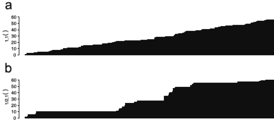
Figure 4.1: Sample trajectories of: (a) standard Poisson process, (b) fPp with parameter \nu = 1/2 . The x-axis is time and the y-axis is the cumulative count of the fractional Poisson process.
